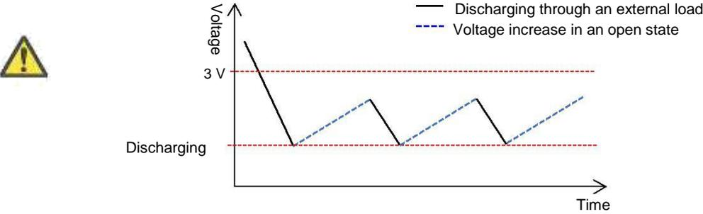
To avoid using the product as described above, **charge it to a voltage equal to or greater than 3 V before starting to discharge.**
